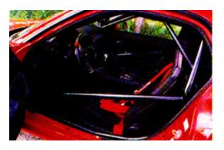
The interior retains most of the stock amenities. For safety, a welded-in chromemoly roll cage, NHRA-approved to 7.50-seconds is on call.
