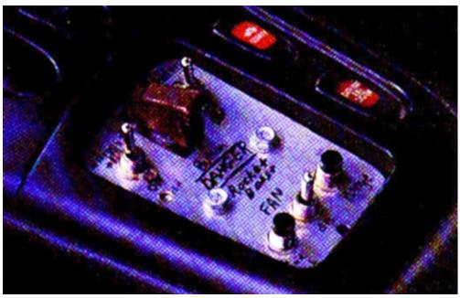
This center consolemounted switch panel commands the Nitrous Express system. It can be easily hidden, adding to the stealth-like aura of the
